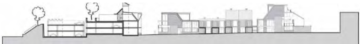
Section showing multi-storey car park wrapped with commercial and residential units (Image source: Source: www.spacetopark.org )
